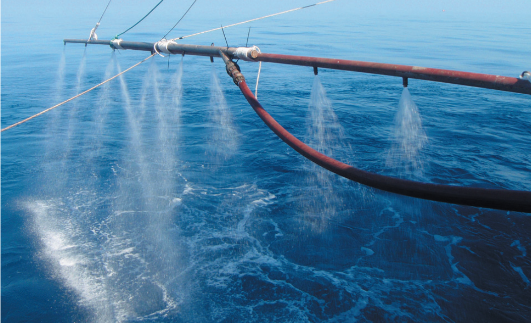
Dispersant spraying from a vessel-mounted spraying arm.
