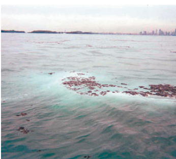
A white plume indicates that the dispersant is not effective on this highly viscous oil.
